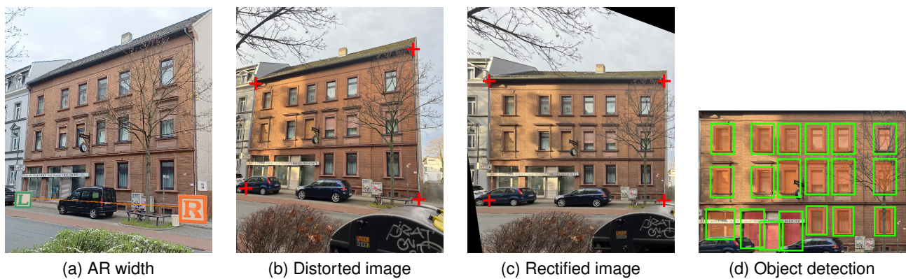
Figure 1: Results of each step of the process. The first figure shows the AR measurement of the facade width. The second figure shows the distorted photo taken by the user with the corner points of the contour. In the third figure the photo was rectified and in the last figure, facade elements have been identified.
