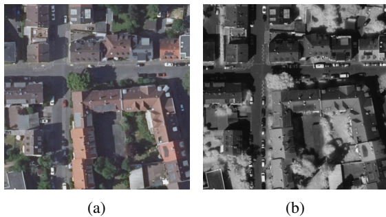
Figure 3: Example RGB (left) and IR (right) pair of aerial images used as input for our training. The imagery was provided by the German Federal Agency for Cartography and Geodesy (BKG).
